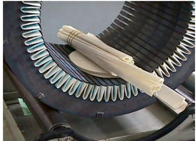
Premium Electrical Steel for improved efficiency, reliability and repairability, C4 coated silicon steel can withstand burnout oven temperature of 500°C (932F) minimum, to insure motors can be rebuilt to original performance.
