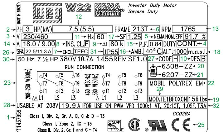
Figure 18 - Nameplate layout for frames 143T to 215T
