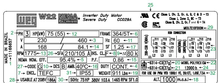
Figure 19 - Nameplate layout for frames 254T to 588/9T
